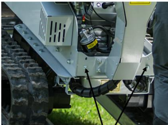
BELT TENSION ADJUSTMENT SCREWS
